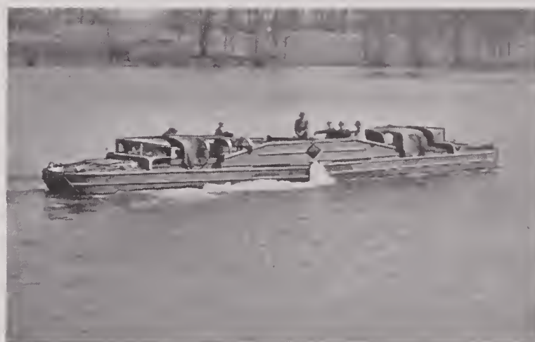
FIGURE 82. DUKWs secured in stern-to-stern tandem for ponton tests.
